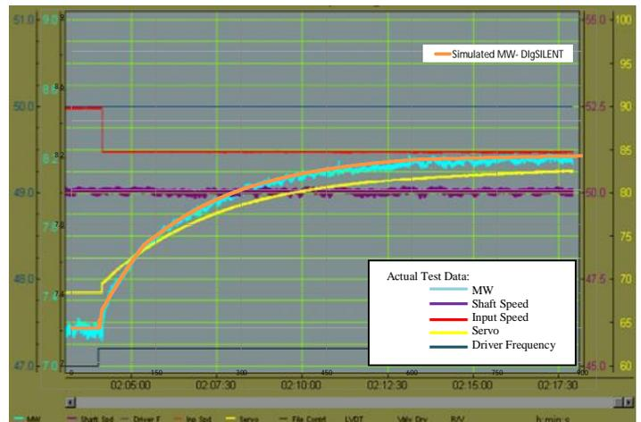
Figure 11. G4: On-line under frequency injection: Simulated vs Test
