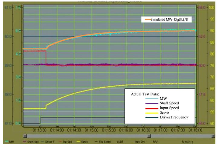
Figure 10. G3: On-line under frequency injection: Simulated vs Test
