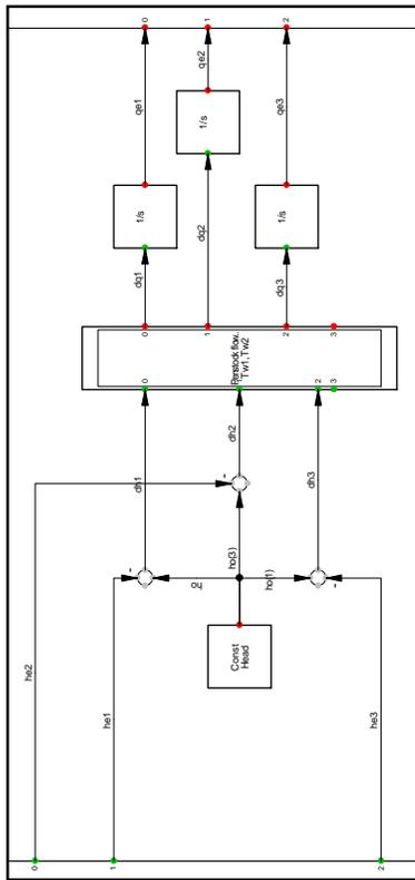
Figure 7. Turbine Model – Common Penstock Model (G2A-1, G2A-2 and G2A-3)
