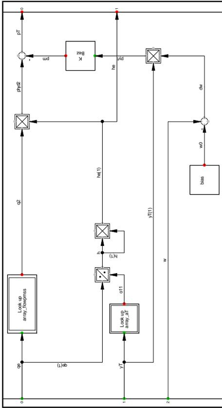
Figure 6. Turbine Model – Shared Penstock (G2A-1, G2A-2 and G2A-3)
