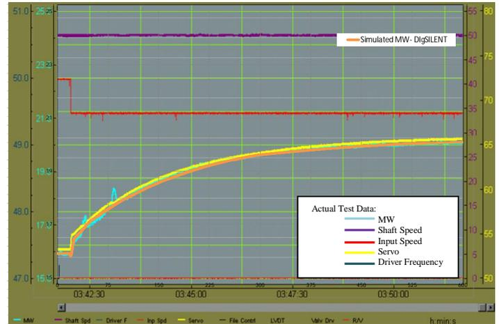
Figure 9. G2A-1: On-line under frequency injection: Simulated vs Test
