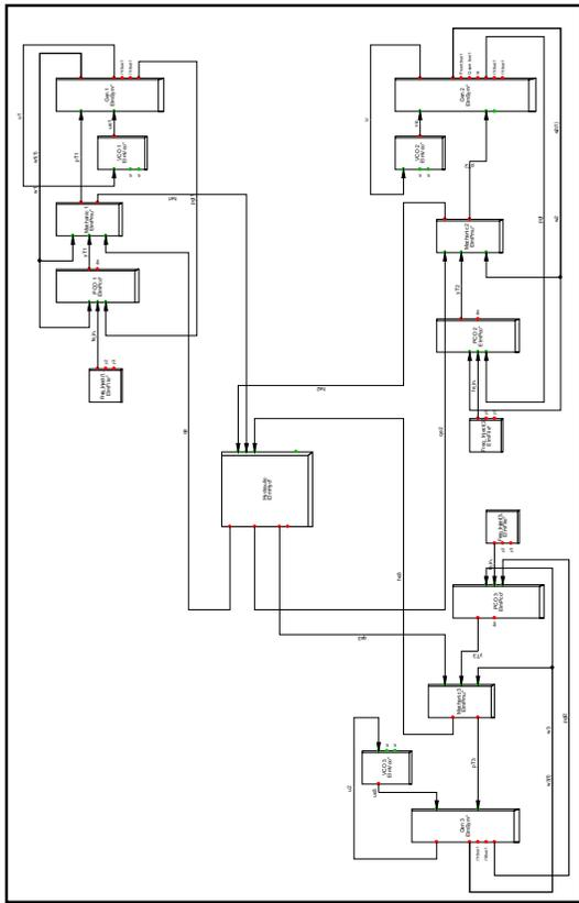
Figure 3. Plant/Frame Model for Shared Penstock Units (G2A-1, G2A-2 and G2A-3)
